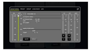
LAST SETTINGS STORED ON DVA MINI G2 (USING DBTECHNOLOGIES AURORA NET SOFTWARE), CAN BE RECALLED LATER ON THE SPEAKER, WITHOUT RDNET REMOTE CONTROL: SIMPLY TURN THE ROTARY "DSP Preset" ON "SERVICE/USER" POSITION.
